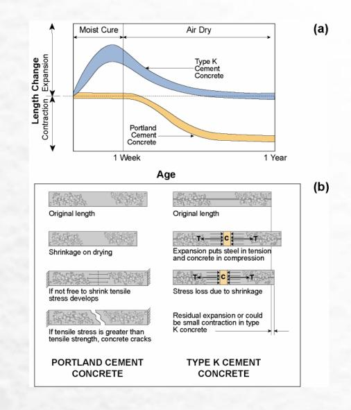
Mixture of portland cement, calcium aluminate cement (with CA is the principal compound), and calcium sulfate.
